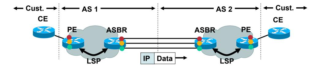
Control plane: No signalling, no labels – interfaces external to AS are pure IP, each ASBR holds its own VRF for the shared VPN
